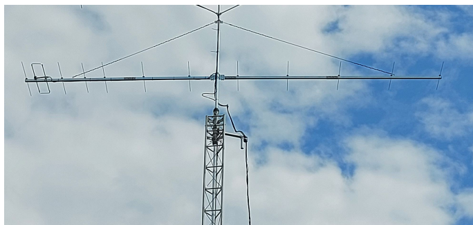
A 12 element low-noise 144MHz LFA Yagi
