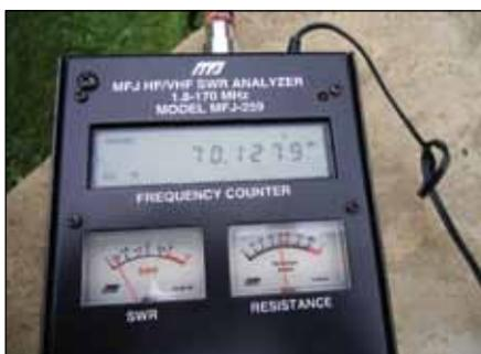
Fig. 7: Resonance, SWR and feedpoint resistance as measured on an MFJ-259
