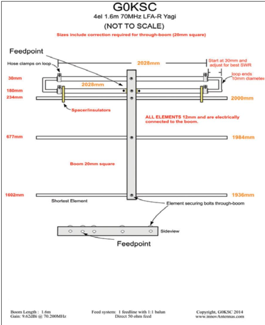
Fig. 4: The antenna construction and measurements.
