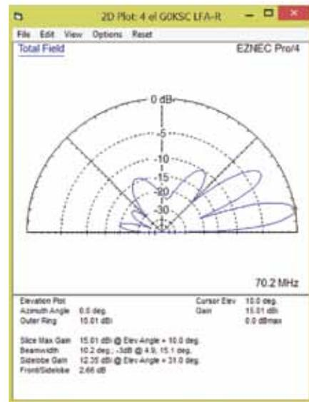
Fig. 3: The elevation plot modelled with the antenna at 6m above average ground – quite different to the free space plot of Fig. 2.
