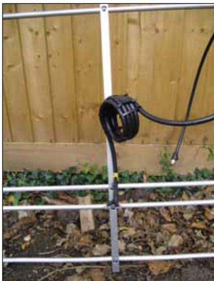
Fig. 6: A coaxial choke at the feedpoint.
