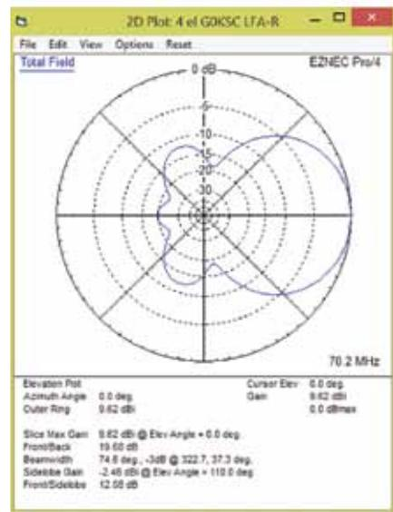
Fig. 2: The elevation free space plot of the antenna.
