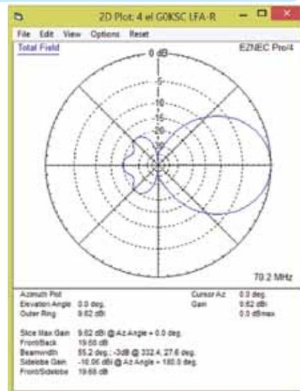
Fig. 1: The azimuth free space plot of the review antenna, modelled in EZNEC.
