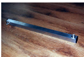
The 2 port 222MHz Power Divider has a flat response for around 11MHz either side of 222MHz
