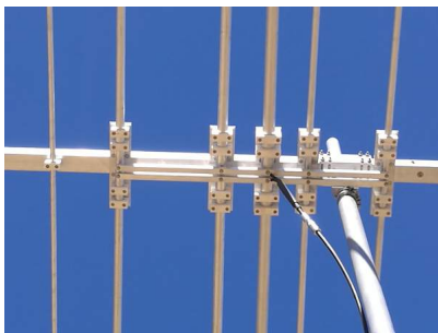
Close-up of the feed arrangement on the XR7 with straight, parrallel lines
